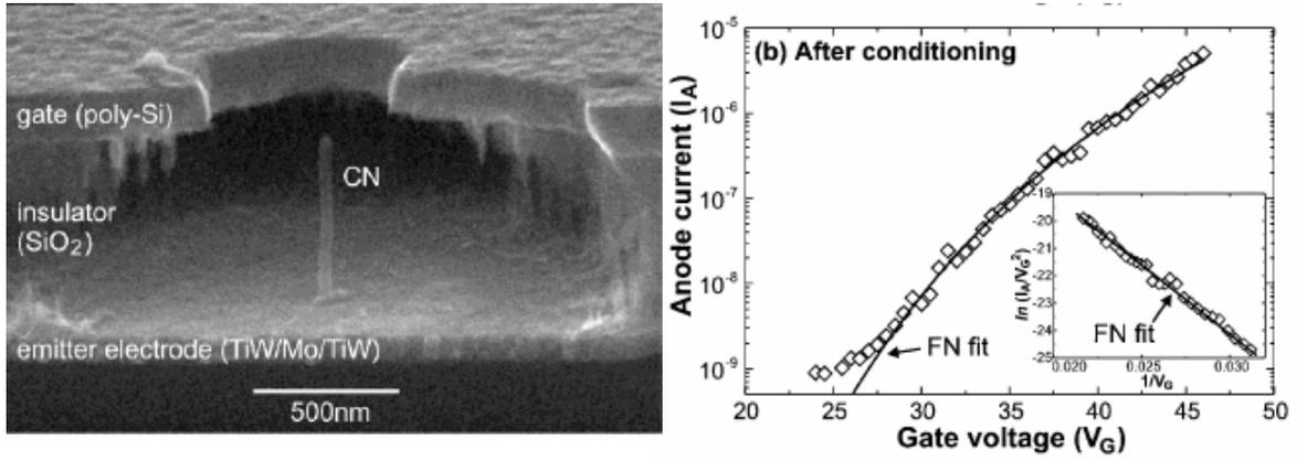
Fig. 1 CNT field emitter and its emission characteristics from [1]
