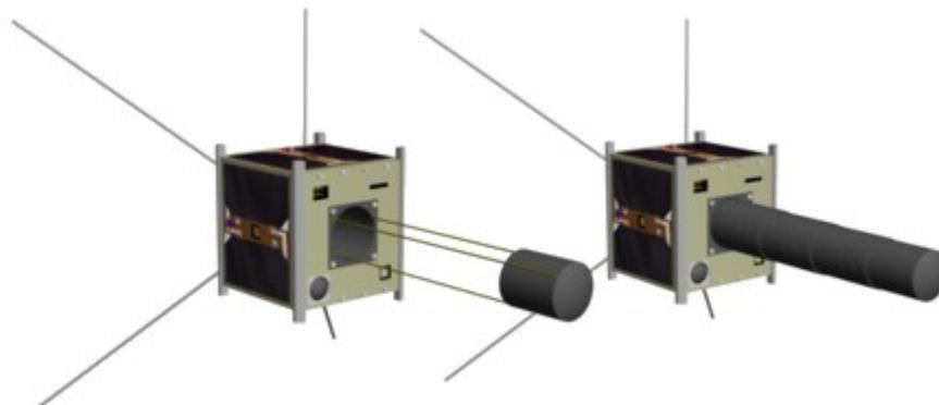
*Figure 2 - DTUsat with two different boom designs
