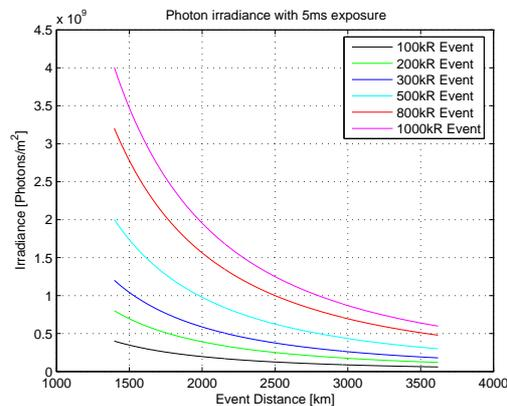
Figure 2: Sprite irradiation intensities for 5ms exposure
