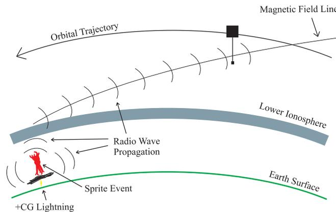
Figure 4: TREC ELF/VLF radio wave reception concept
