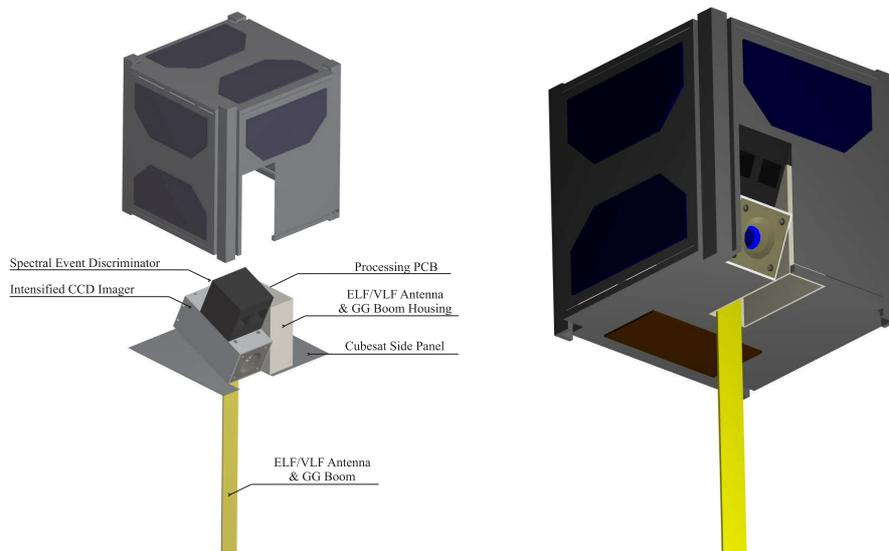
Figure 7: CAD rendering of TREC implemented on CubeSat platform
